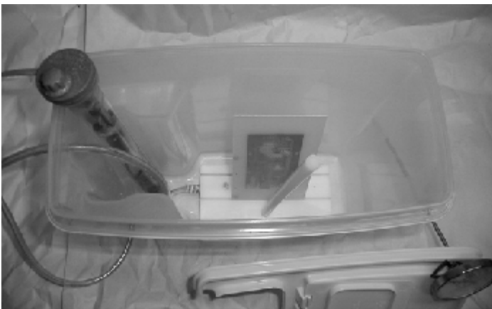
Figure 5-8: Inside view of etchant tank
